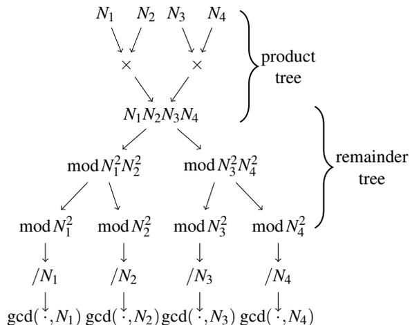
Figure 1: **Computing all-pairs GCDs efficiently** — We computed the GCD of every pair of RSA moduli in our dataset using an algorithm due to Bernstein [7]: First, compute the product of all moduli using a product tree, then use a remainder tree to reduce the product modulo each input. The final output is the GCD of each input modulus with the product of all the other moduli.
