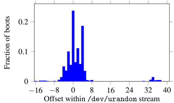
Figure 6: **Predictable output from `urandom`**—When we disabled entropy sources that might be unavailable on a headless or embedded device, the Linux RNG produced the same predictable stream on every boot. The only variation we observed over 1,000 boots was the *position* in the stream where `sshd` read from `urandom`.
