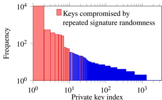
Figure 4: **Vulnerable DSA keys for one SSH device** — We identified 18,684 SSH DSA keys that appeared to have been generated by Gigaset DSL routers, of which 16,575 were repeated at least once. Shown in red in this log-log plot are 12,378 keys further compromised due to repeated DSA signature values. The more commonly repeated DSA keys were more likely to be compromised by repeated signatures, as they are more likely to have collisions between hosts in subsequent scans.
