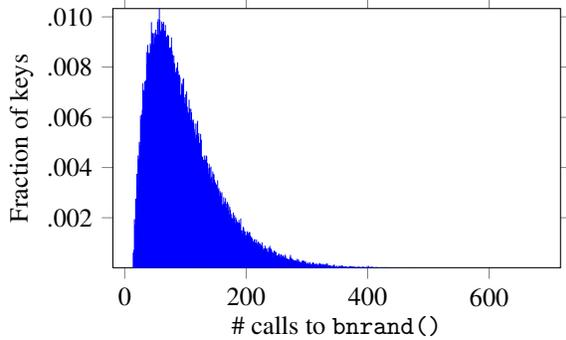
Figure 7: **Calls to bnrnd() during key generation** — Every time OpenSSL extracts randomness from its internal entropy pool using bnrnd(), it mixes the current time in seconds into the pool. This histogram shows the number of calls for 100,000 1024-bit RSA key generation operations. Both the average and the variance are relatively high due to the probabilistic procedure used to generate primes.
