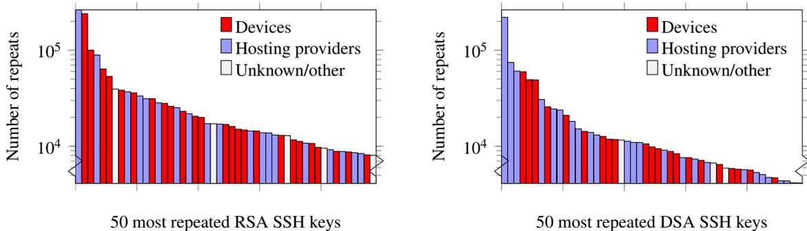
Figure 2: **Commonly repeated SSH keys** — We investigated the 50 most repeated SSH host keys for both RSA and DSA. Nearly all of the repeats appeared to be due either to hosting providers using a single key on many IP addresses or to devices that used a default key or generated keys using insufficient entropy. Note log scale.
